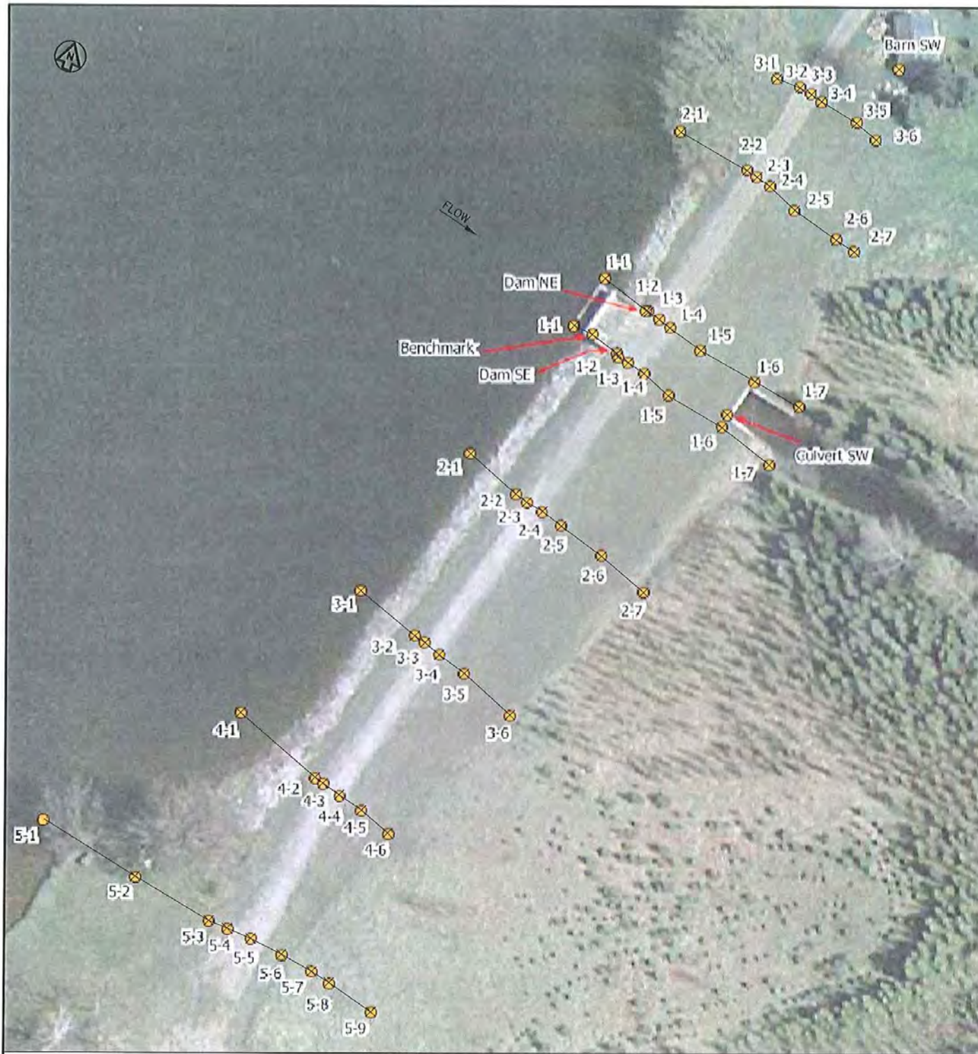
DAM - AS CONSTRUCTED CROSS SECTION LOCATIONS SCALE 1:300
