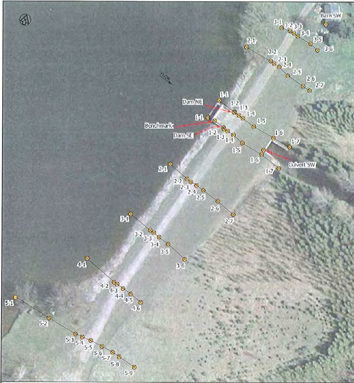
DAM - AS CONSTRUCTED CROSS SECTION LOCATIONS SCALE 1:300
