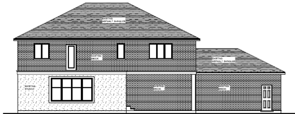
EXISTING REAR ELEVATION
