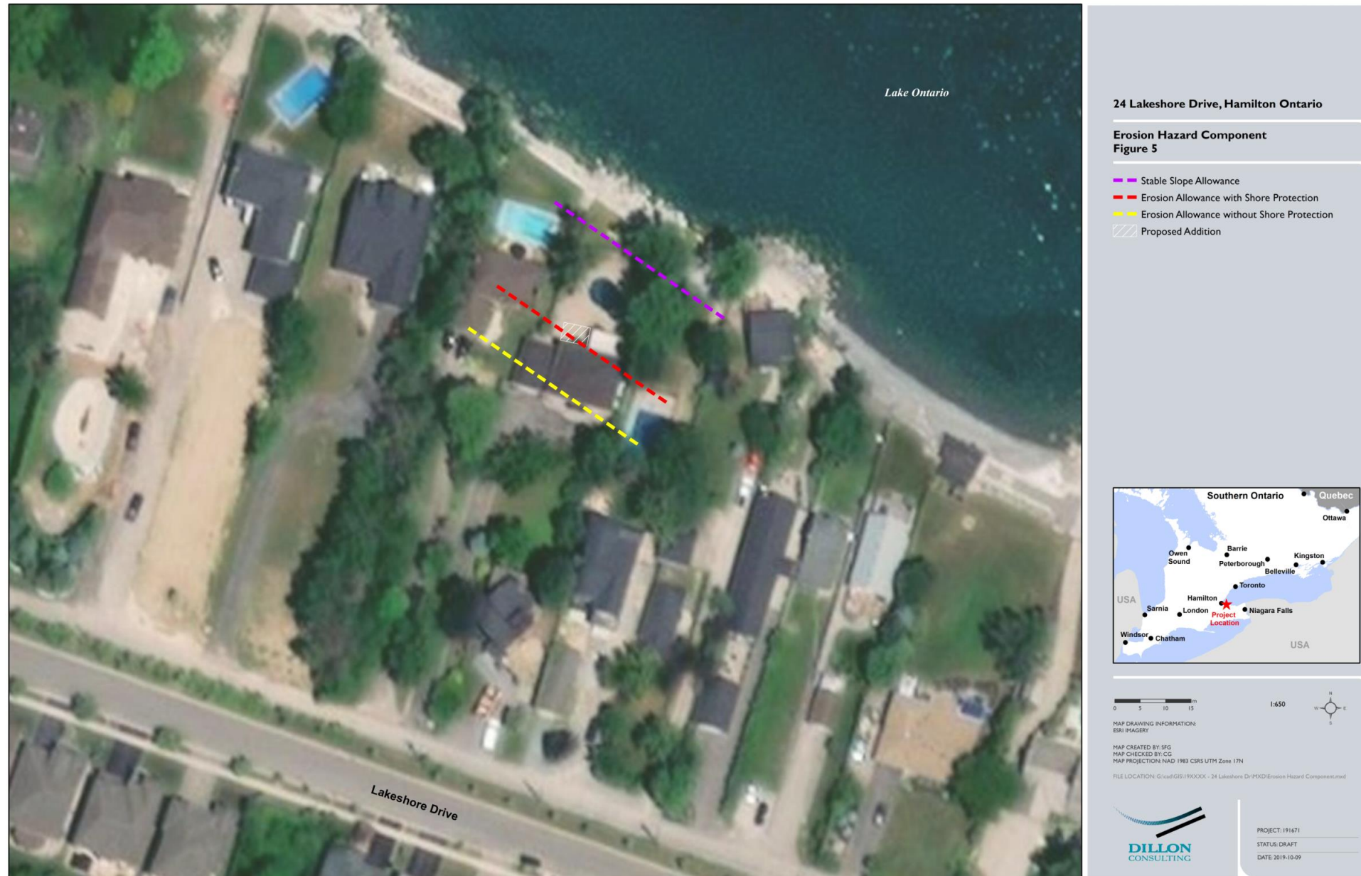
Figure 5 – Plan View of Erosion Hazard Components at 24 Lakeshore Drive
