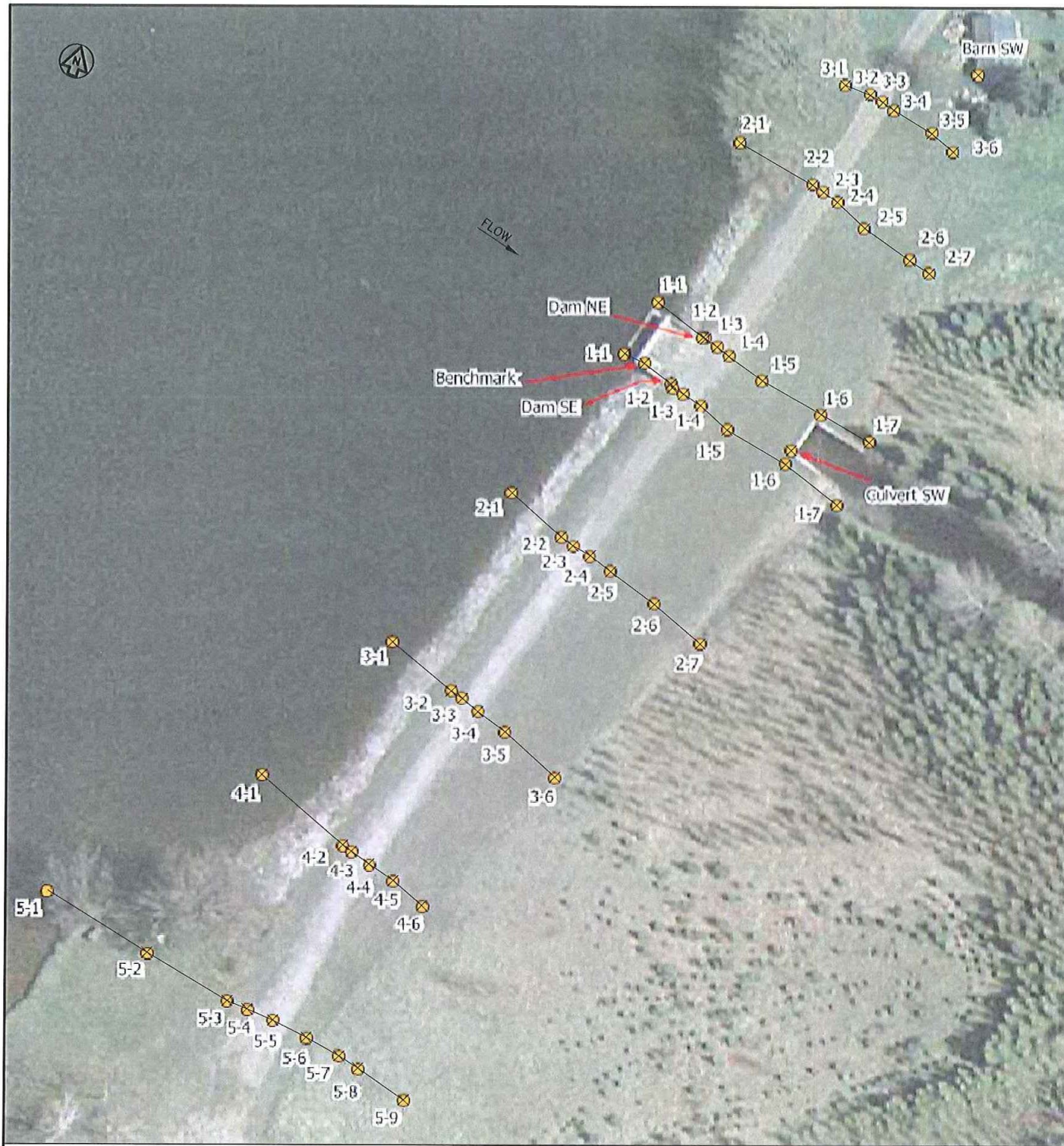
DAM - AS CONSTRUCTED CROSS SECTION LOCATIONS SCALE 1:300
