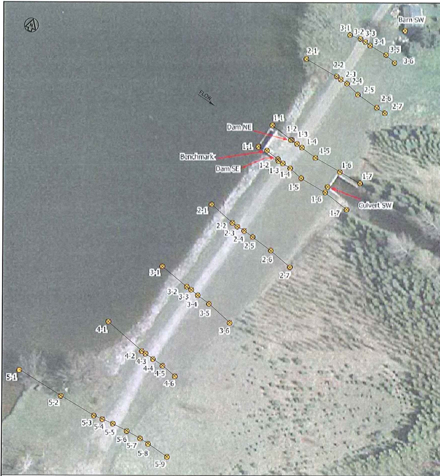
DAM - AS CONSTRUCTED CROSS SECTION LOCATIONS SCALE 1:300
