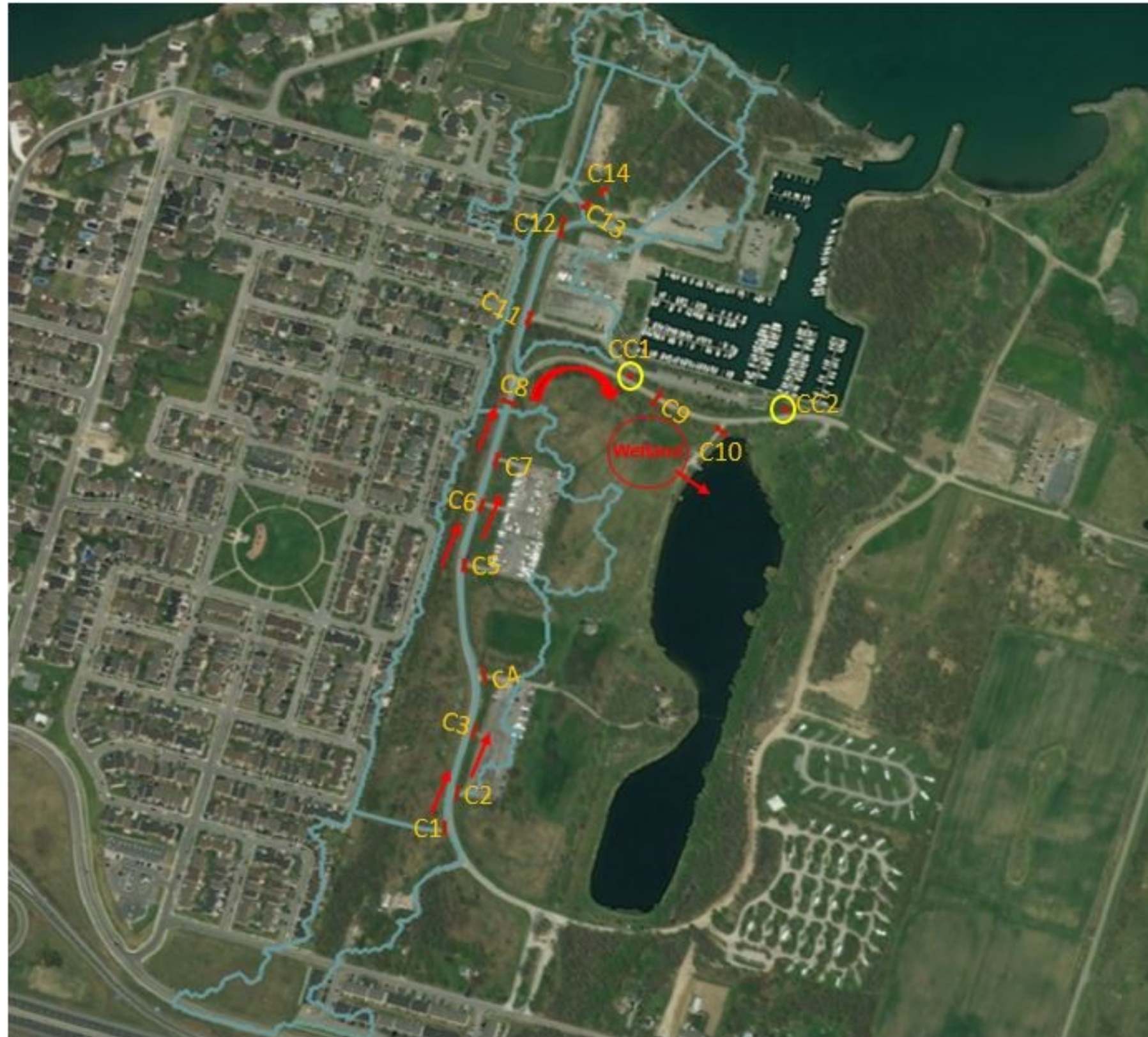
Figure 20: Flow Direction in Proposed Design Condition
